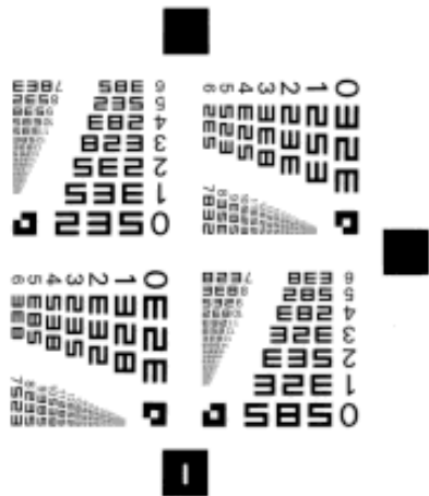
Fig. 26 RIT Alphanumeric test target. It consists of lines of block letters. During inspection, an observer must recognize letters, rather than detect resolved line pairs. Can be used for "legibility tests."
