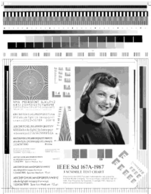
Fig. 22 IEEE Std 167A-1987 facsimile test chart designed for use with facsimile machines. It is produced photographically and includes gray-scale bars, test, rules, and a continuous-tone image. It also incorporates traditional line-pair patterns.
